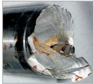
Pump Shaft Fatigue Failure
