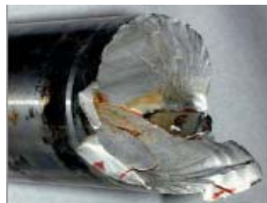
Pump Shaft Fatigue Failure.
